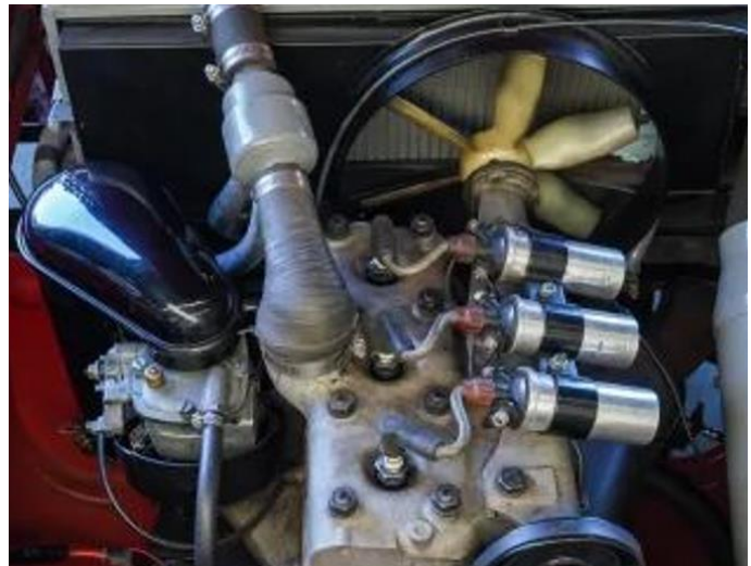
1000cc 3-cyl two-stroke. Twice as much optional.
