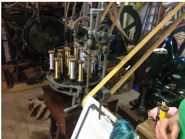
All the equipment runs on line shafts and belts.
